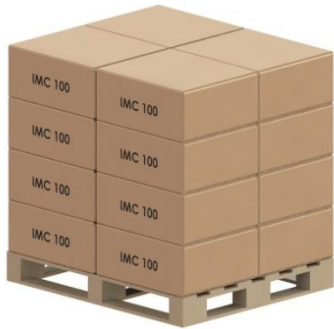
IMC100 4 Cartons per Layer 4 Layers per Unit Load max 16 Cartons per Unit Load max 1 Layer with Pallet 367mm
