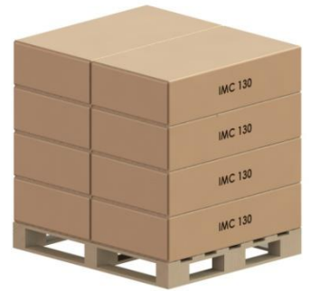
IMC130 2 Cartons per Layer 4 Layers per Unit Load max 8 Cartons per Unit Load max 1 Layer with Pallet 367mm
