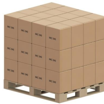
IMC045 16 Cartons per Layer 3 Layers per Unit Load max 48 Cartons per Unit Load max 1 Layer with Pallet 437mm
